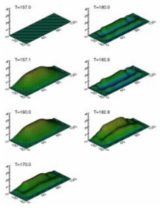
Figure 2: Slip distribution on the fault plane obtained by viscoelastic inversion. Plate motion effects are not included.
