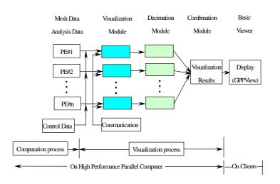
Figure 1: The parallel framework of visualization subsystem in GeoFEM
