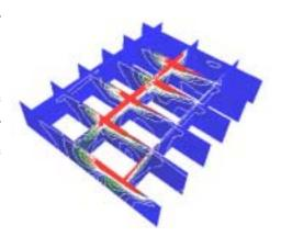
Figure 2: Cross-sectioning for large dataset with 456,365 nodes. Equivalent scalar values of stress are mapped to colors with isolines. (Data courtesy of Mikio Iizuka in GeoFEM)
