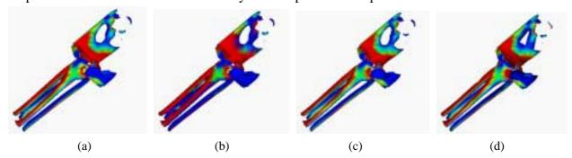
Figure 6. Simplifying interval volume of mechanical part. (a) Original (6,706 patches); (b) 50% patches reduced by accounting for geometry only (r = 0.0); (c) 50% patches reduced by optimized combination of color/geometry deterioration (r = 0.63); (d) 50% patches reduced by accounting for color only (r = 1.0)
