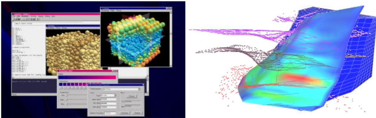
Figure 6: *Left:* The LSMearth micro-scale modelling software system developed at QUAKEs showing a system of particles representing a rock structure being subjected to compression. *Right:* The GeoFEM macro-scale software system developed at RIST by the GeoFEM group showing a large scale simulation of a subduction fault zone.
